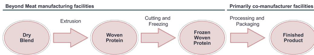
First, a dry blend containing our pea protein is combined within our manufacturing facility. The dry blend then enters our extruder, where both water and steam are added. We then use a combination of
